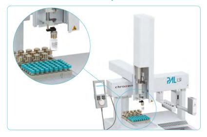
ChroZen PAL systems can reach any three dimensional position within its working area. It is able to transport vials to read barcodes or to transfer the vials into temperature controlled modules like the agitator for heating samples or the peltier stack for cooling them down to 4 °C.
