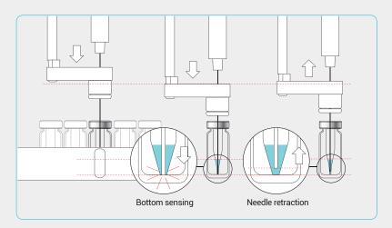
Bottom sensing makes sure that small volume can be injected out of a little µL of sample.(3 injections of 1 µL out of 5 µL sample)
