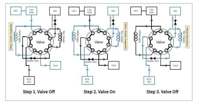
Fig 2. switching time setting of 10-port valve
