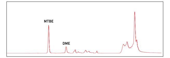
Fig 6. chromatogram of gasoline sample
