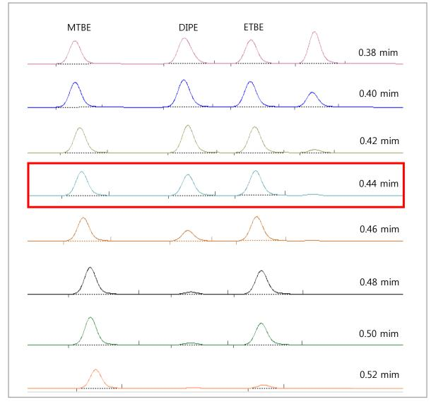
Fig 3. detection by valve switching time using D4815 valve timing mix standard (47212)
